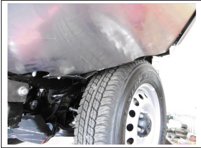
Figure 14. Liner trimmed to fit
